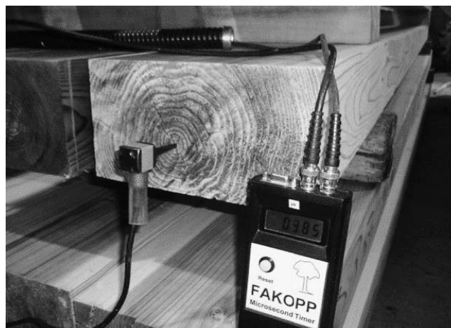
Figure 1.—Placement of sensors for stress wave test.
