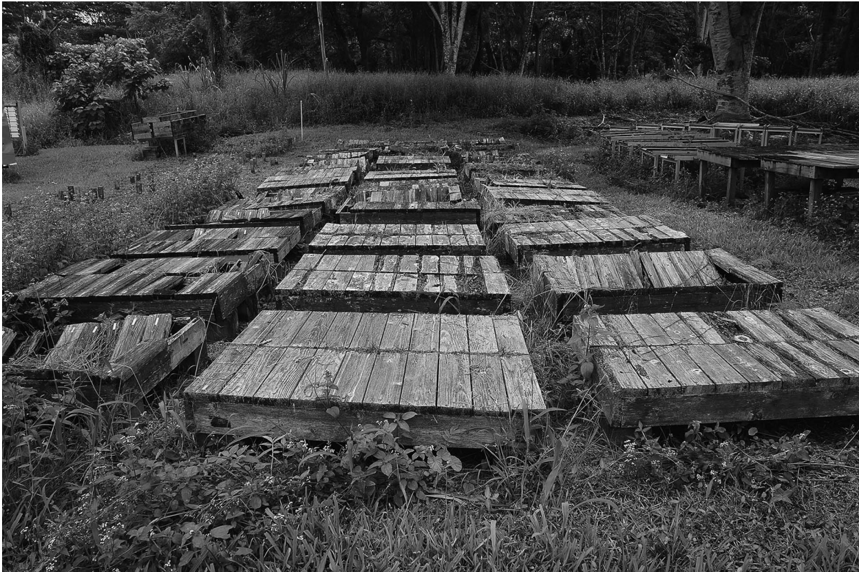
Figure 1.—Decking test units at the Kipuka test site in Hawaii after 7 years of exposure.
