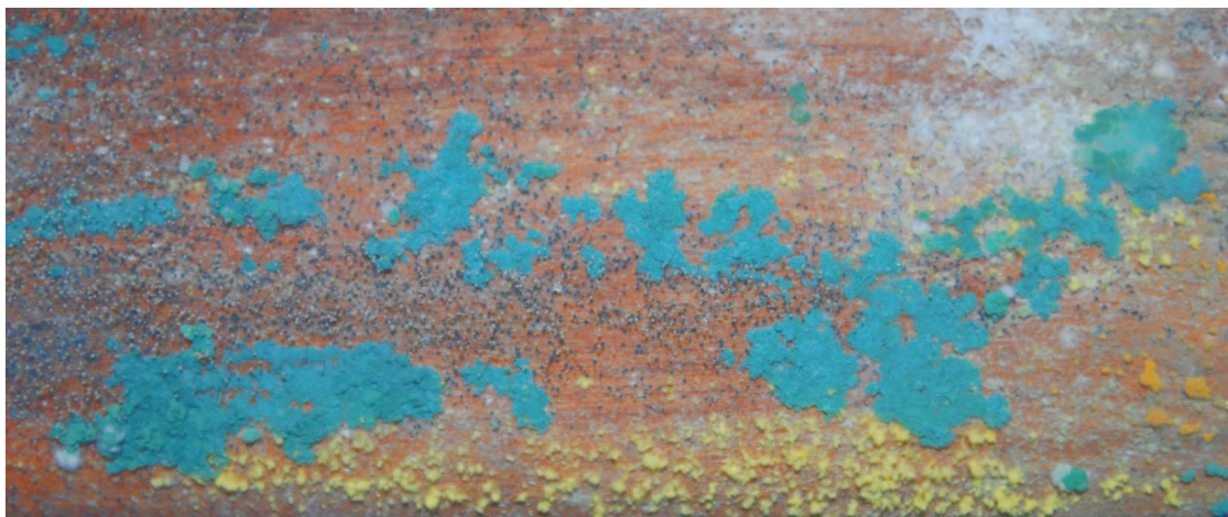
Figure 3.—Colonization and growth of fungal structures after mixed cultures of Ophiostoma sp., Eurotium sp., and Phialocephala sp. were applied on Nothofagus obliqua . (Color version is available online.)
