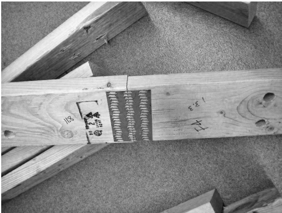
Figure 1.—F4 test specimen after fabrication.
