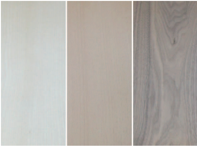
Figure 1.—Appearance of maple (left), beech (middle), and walnut (right) wood before coating application. (Color version is available online.)
