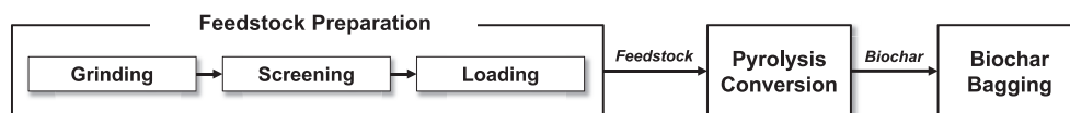
Figure 3.—Cost elements of the entire pyrolysis operation from feedstock preparation to packaging the final product.
