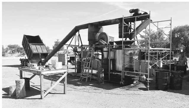
Figure 1.—The Biochar Solutions Inc. mobile pyrolysis system field-deployed and evaluated in this study.
