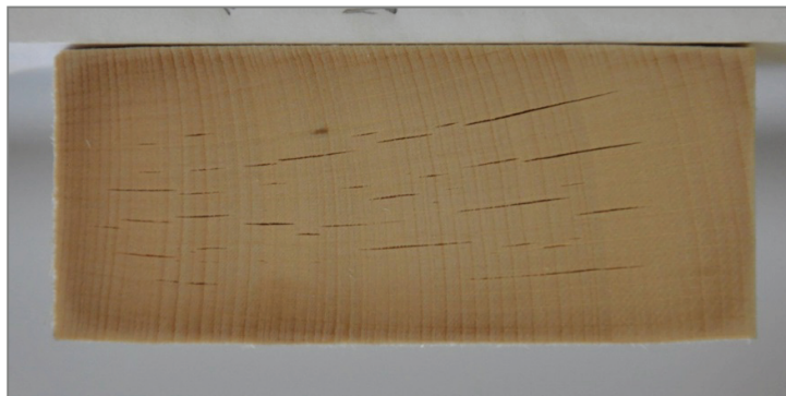
Figure 1. Cross section of a sample dried at a high drying gradient for three hours– deformation, discoloration and checks are well apparent (red rectangle is original cross section)
