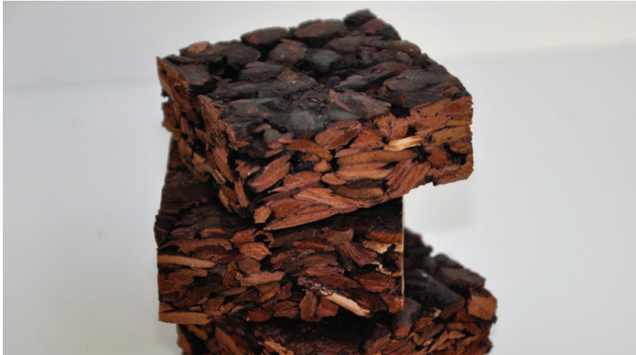
Figure 2. Tannin-resin bonded bark insulation panel (thickness = 20 mm, density = 400 kg/m 3 )
