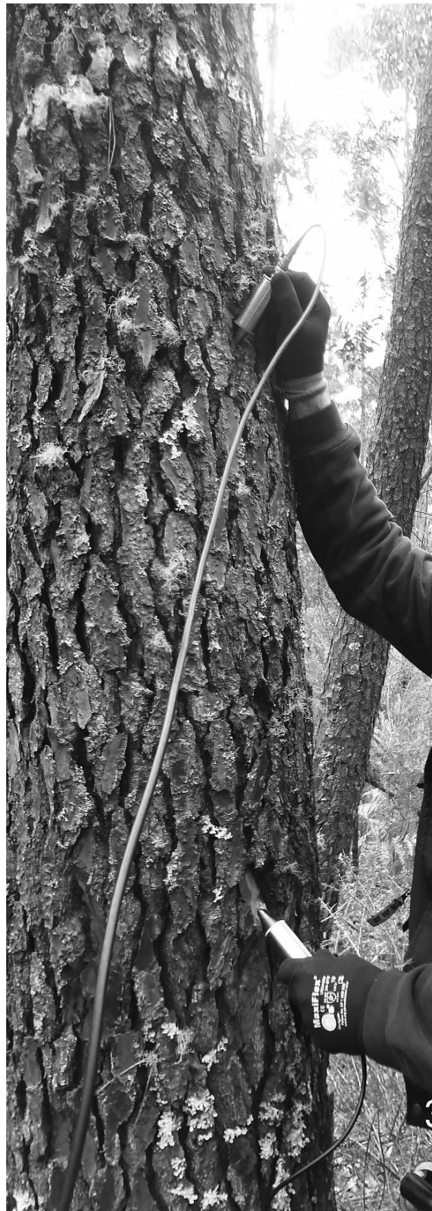
Figure 1.—Placement of transducers for ultrasonic testing of trees.
