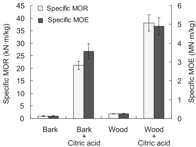
Figure 3.—Bending properties of the wood-based moldings. MOR = modulus of rupture; MOE = modulus of elasticity.
