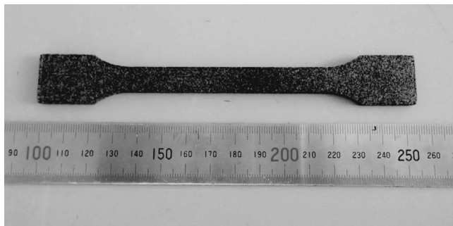
Figure 1.—Wood-based molding bonded with citric acid.
