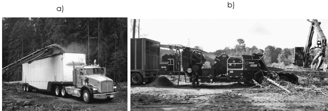
Figure 1.—(a) Conveyor-fed loading method into a chip van in a grinding operation; (b) horizontal blowing of wood chips into trailers.
