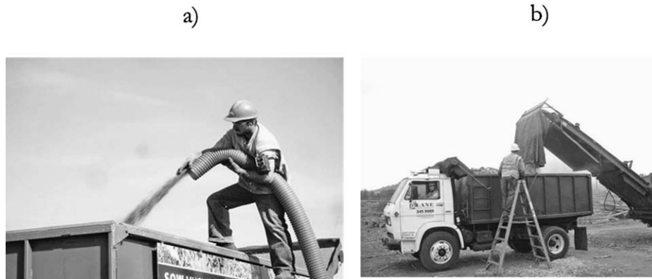
Figure 4.—(a) Near-vertical high speed blowing of grindings during truck loading; (b) conveyor-fed truck loading.
