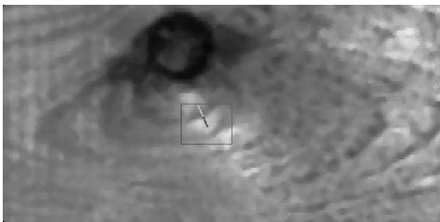
Figure 5.—Both grain angle normals (light and dark gray lines inside the square) correspond to the same local grain direction.
