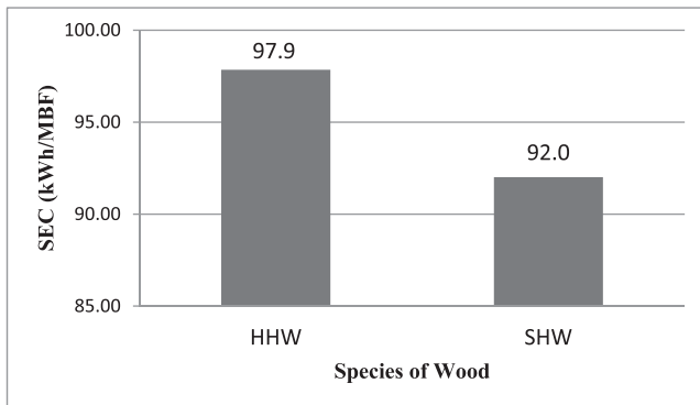
Figure 4.—Specific energy consumption (SEC) in kilowatt hours (kWh) per thousand board feet (MBF) for hard hardwoods (white ash, hickory, hard maple, red oak, and white oak) and soft hardwoods (black birch, black cherry, soft maple, and yellow-poplar).
