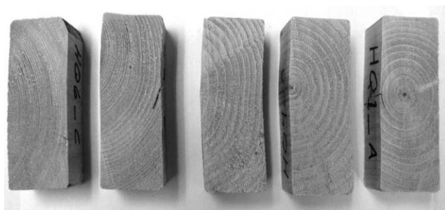
Figure 2.—Typical representative cross sections from five spruce-pine-fir south (SPF-s) 2 by 4s.
