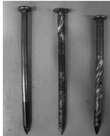
Figure 1.—Photo of nails tested (from left) 8d common, 8d annular, and 8d helical.
