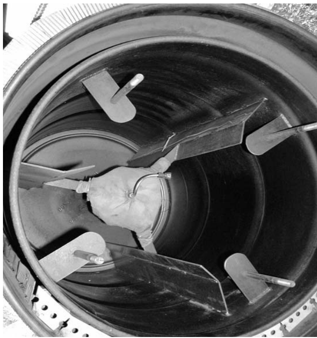
Figure 2.—Inside of drying chamber. Air leaves through cloth filter at center and passes through 2-cm tube to back of photo. Air enters through small curved tube at center. Tube is concentric with exhaust tube.
