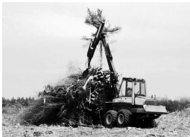
Figure 3.—Residue forwarding from stump area to the landing by a cut-to-length forwarder in this study.
