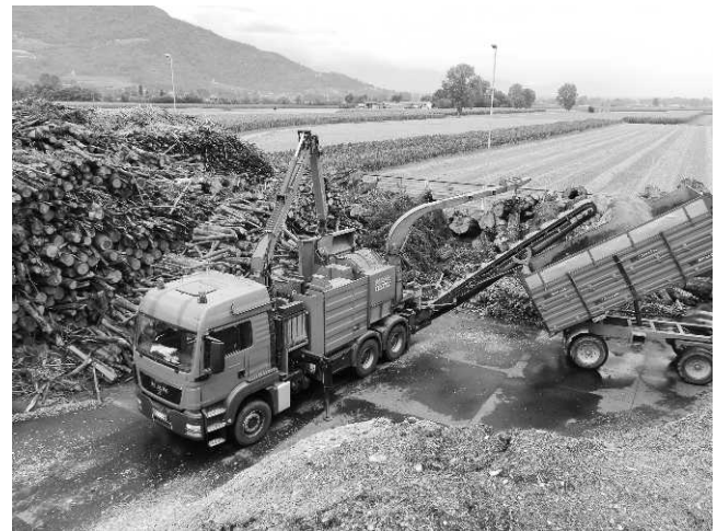
Figure 2.—The industrial chipper truck using the belt conveyor discharge system.
