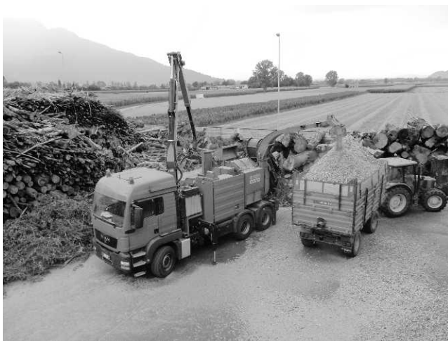
Figure 1.—The industrial chipper truck using the blower discharge system.
