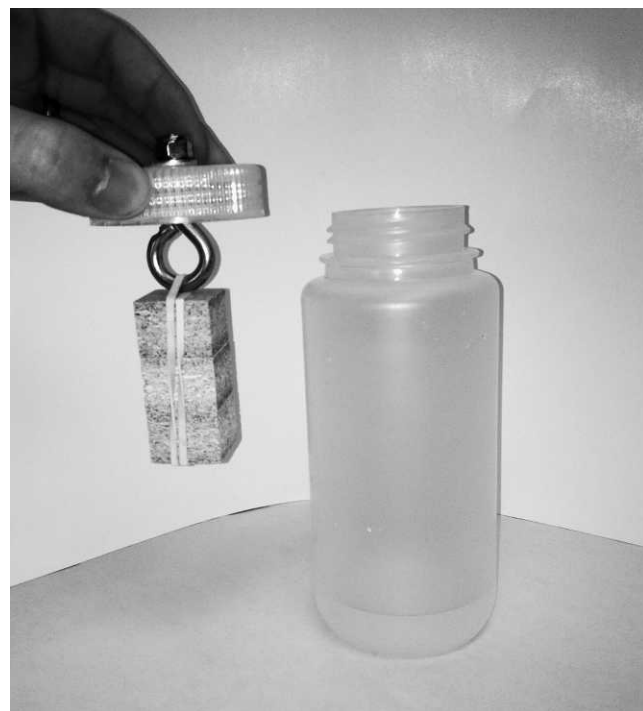
Figure 2.—Sample set-up for modified EN 717-3 method (ÖNORM, 1996).
