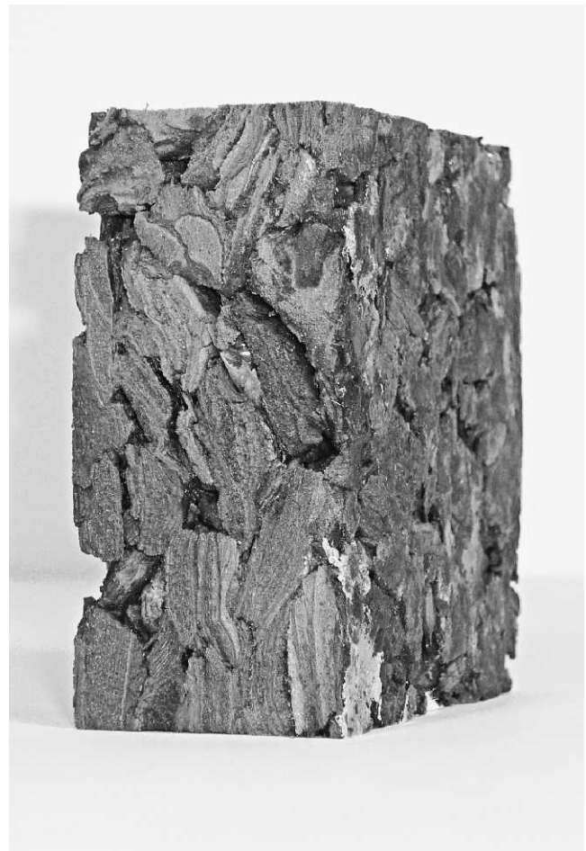
Figure 1.—Bark-based insulation panel (thickness, 20 mm; density, 400 kg/m 3 ; particle size, 30 mm > x_4 ≥ 13 mm).
