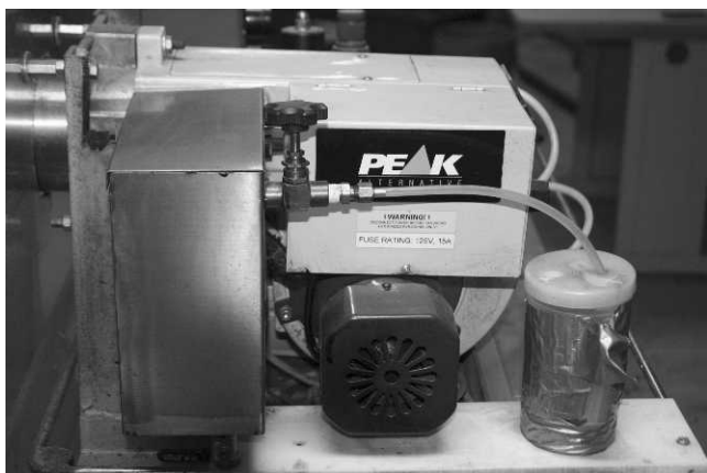
Figure 1.—Side view of the Peak burner showing the small diesel fuel container on the right with a control valve on the line entering the main tank that holds the bio-oil.
