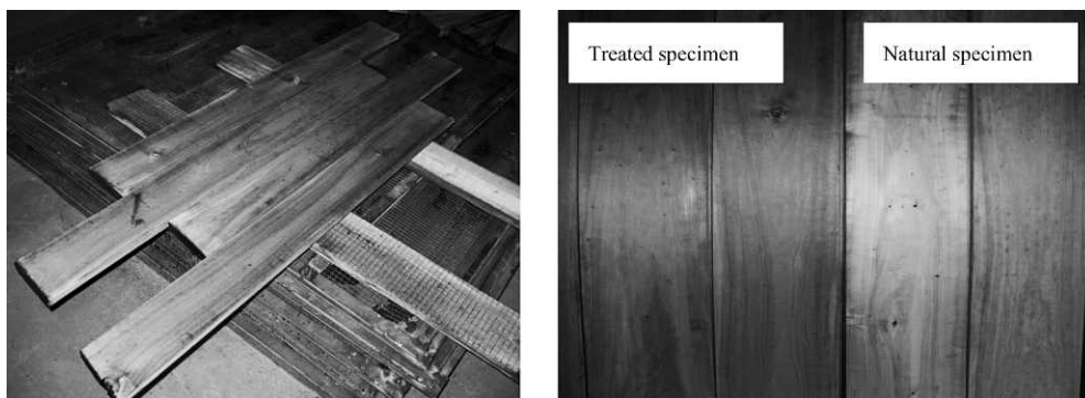
Figure 7.—(Left) Treated specimen and (right) comparison between treated and untreated specimens.
