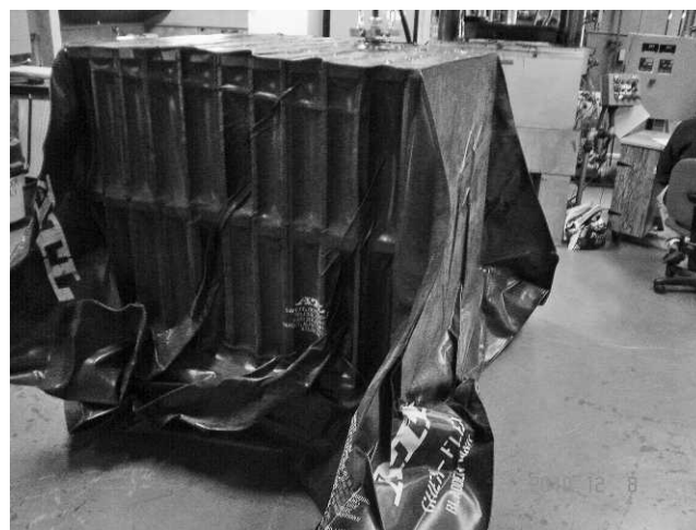
Figure 2.—Collapsed flexible container after vacuum was applied to the system.
