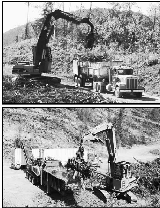
Figure 1.—The slash forwarding system (left) transports forest residues in end-dump trailers to a concentration yard, where they can be stockpiled and ground into large chip vans. The in-woods grinding system (right) processes residues on the treatment unit and transports hog fuel to the concentration yard, where it is stockpiled and loaded into chip vans with a front-end loader.
