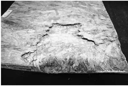
Figure 3.—Oriented strand board from aspen after 5 years of exposure at 45°.
