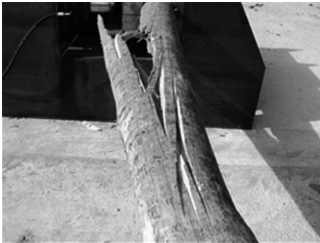
Figure 5.—Failure by tension.
