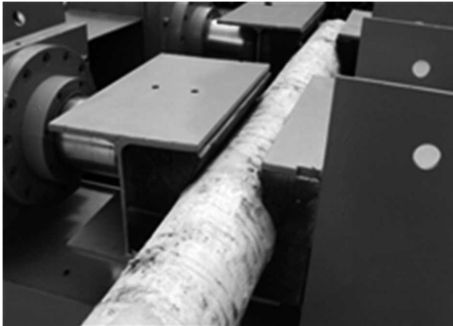
Figure 3.—An example of a pole rigidly clamped.
