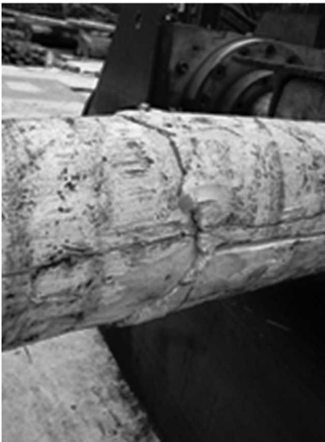
Figure 6.—Failure by compression.
