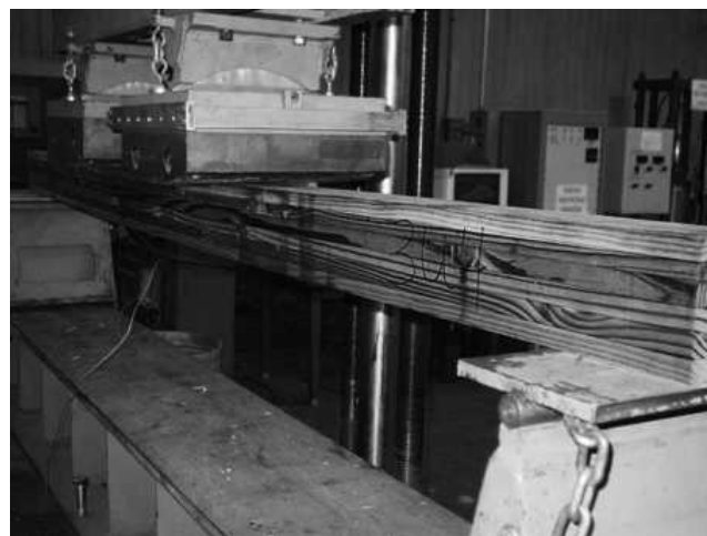
Figure 2.—Testing setup for the flexural tests of laminated beams (Composition D) consisting of four decommissioned pentachlorophenol-treated southern pine utility pole wood plies (middle) and two untreated southern pine virgin wood plies (top and bottom).
