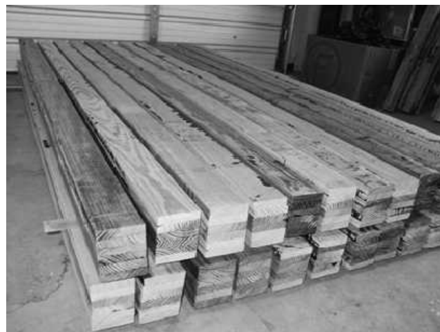
Figure 1.—Some of the laminated beams made of pentachlorophenol-treated southern pine utility pole wood and untreated virgin wood.
