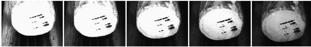
Figure 9.—Five consecutive images of a log end surface acquired using various camera exposure times (i.e., 650, 500, 350, 250, and 150 \mu s). The same light intensity was used when acquiring all images. The coded number is 545.
