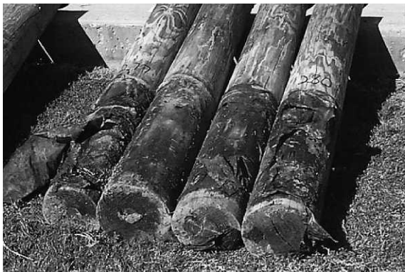
Figure 11.—Typical performance of fluoride paste (left) and copper borate paste (right) treatments with no decay after 41 months of exposure in American Wood-Preservers' Association Hazard Zone 4.
