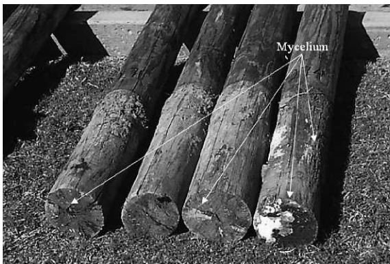
Figure 12.—Performance of fluoride (left) and boron (right) rod treatments after 41 months of exposure in American Wood-Preservers' Association Hazard Zone 4.
