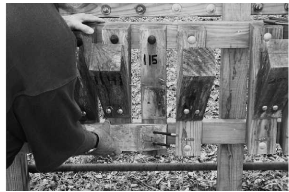
Figure 5.—Post-rail units exhibiting poor (left) and excellent (right) performance after 44 months of exposure.
