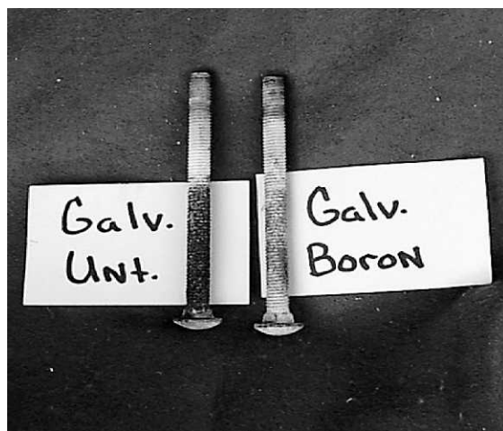
Figure 9.—Corrosion of galvanized bolts was much less in those that had been dipped in BoraCare (1:1) prior to use (left) and a corroded galvanized fastener in an oak test unit (right) after 44 months of exposure.
