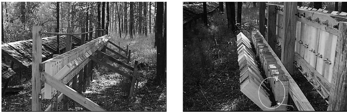
Figure 2.—Post-rail units exposed on vertical test fences at the Dorman Lake test site in American Wood-Preservers' Association Hazard Zone 4 (units on right have preservative paste applied to the joint [circle]).
