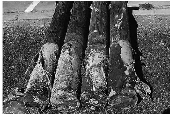
Figure 11.—Typical performance of fluoride paste (left) and copper borate paste (right) treatments with no decay after 41 months of exposure in American Wood-Preservers' Association Hazard Zone 4.
