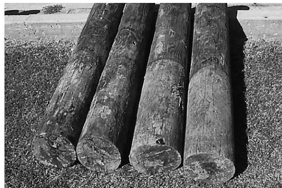
Figure 12.—Performance of fluoride (left) and boron (right) rod treatments after 41 months of exposure in American Wood-Preservers' Association Hazard Zone 4.
