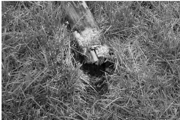
Figure 10.—Typical failed untreated pole stub after 41 months in service in American Wood-Preservers' Association Hazard Zone 4.
