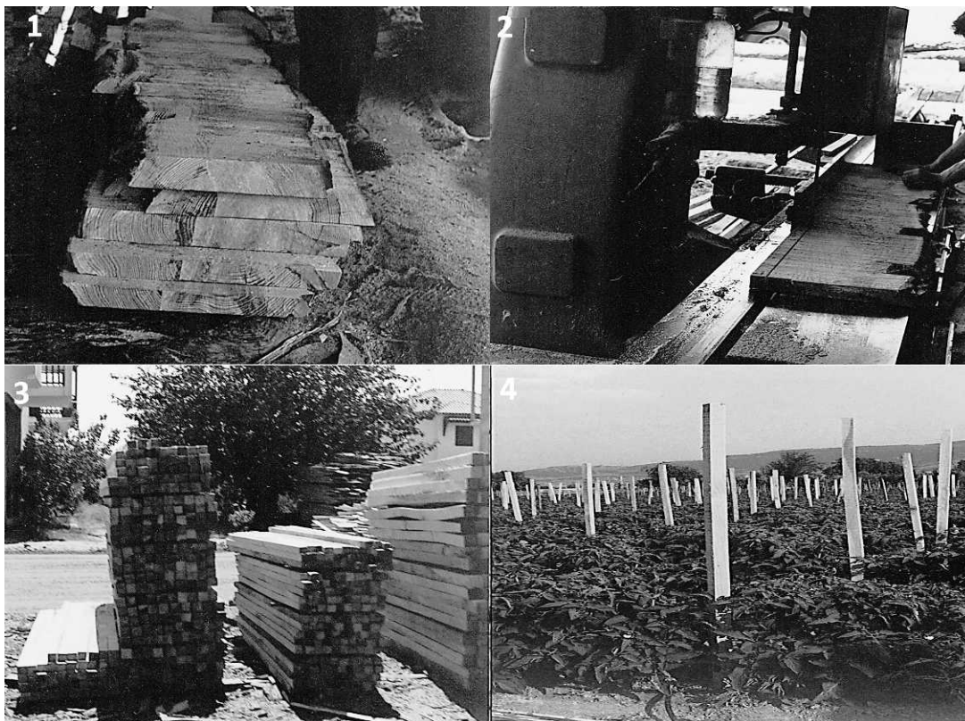
Figure 1.—(1) Lumber produced at the local sawmill from deresinated Pinus halepensis logs; (2) lumber sawing to produce posts; (3) produced posts in different dimensions stored at the sawmill yard; (4) the posts used to support tomatoes in field cultivation.
