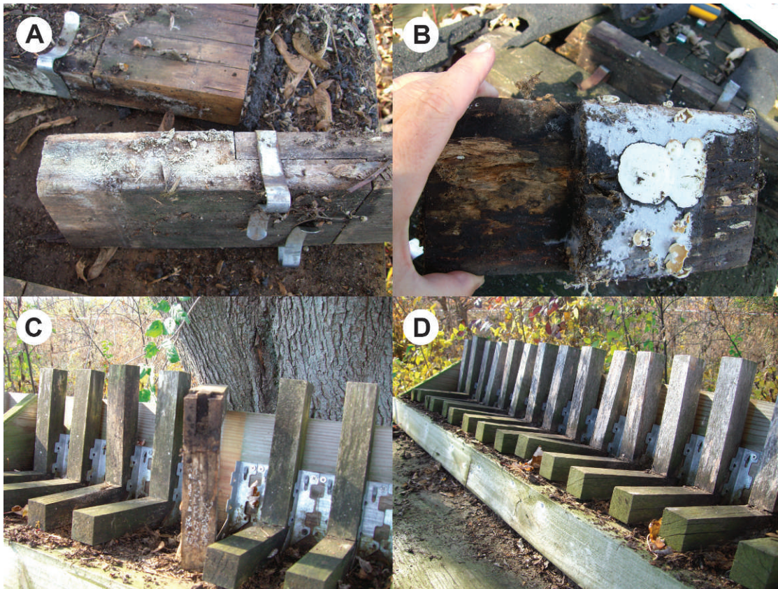
Figure 3.—Fungal fruiting bodies and mycelium on white pine lap joint (A), maple lap joint (B), white pine L joints (C), and maple L joints (D).
