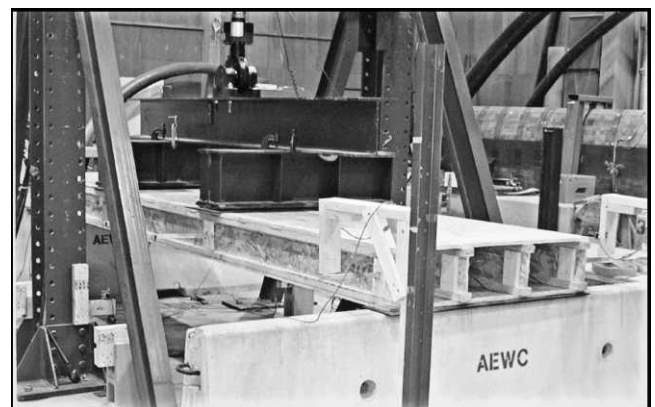
Figure 5.—Panel in four-point bend setup.
