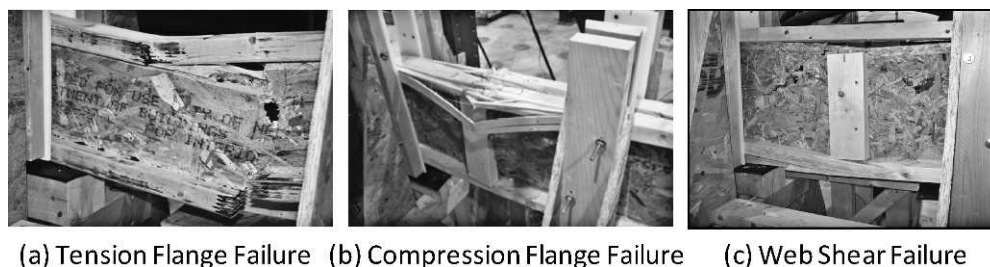
Figure 9.—I-joist failure modes.
