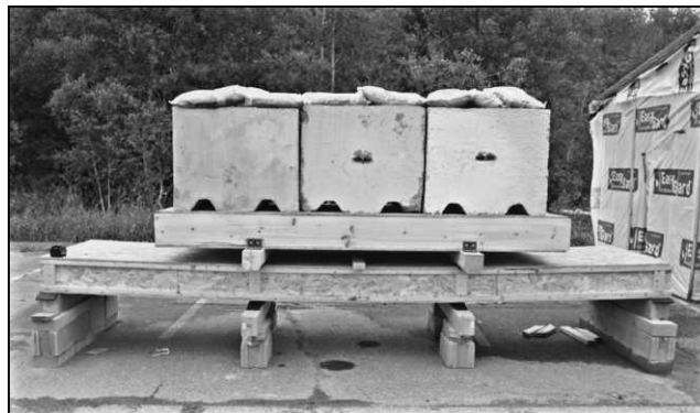
Figure 6.—Creep test prior to sheltering specimen.
