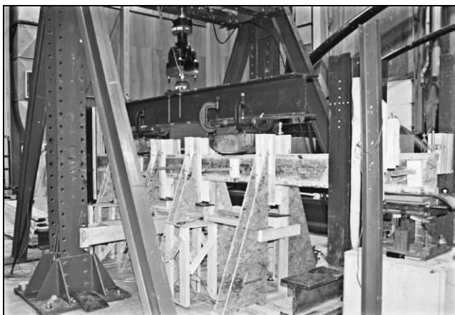
Figure 4.—I-joist specimen in four-point bend setup.
