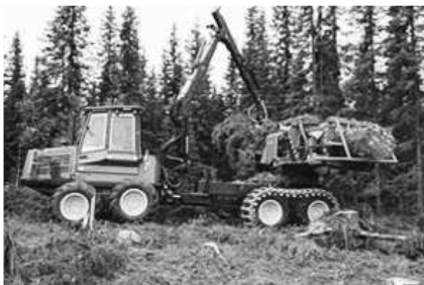
Figure 1.—John Deere 1490D Slash Bundler (courtesy of John Deere). The machine features a bundling unit with a forwarder for mobility.
