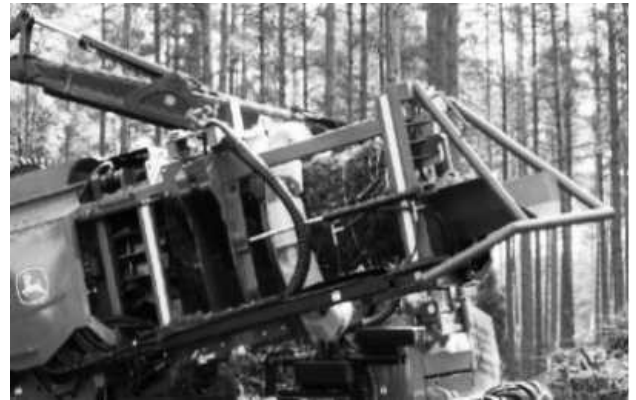
Figure 2.—John Deere B380 Bundler unit, which makes a continuous compressed residue log (bundle).
