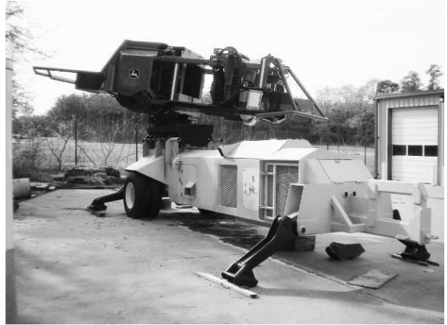
Figure 5.—Trailer-mounted B380 bundling unit.
