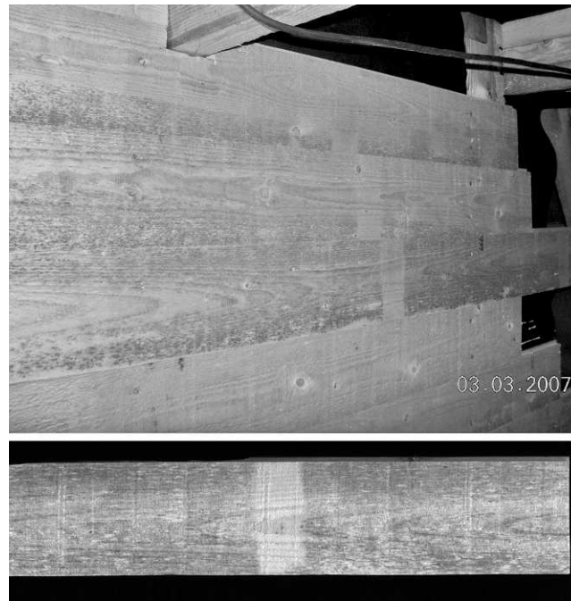
Figure 1.—Mold growth on a wall of tongue and groove boards of Norway spruce in an unheated outdoor carport after approximately one year's usage. Note the brighter areas without mold where stickers had been placed during kiln drying.
