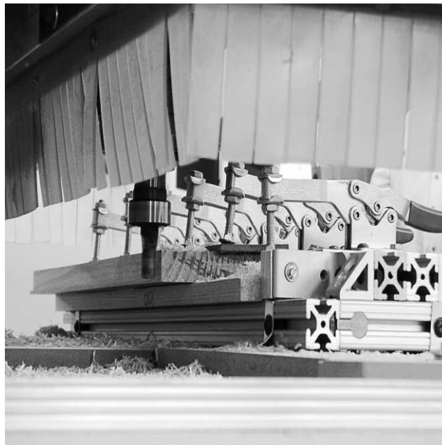
Figure 1.—Tool wear test conditions: router table, single insert tool holder, specimen fixture, and test specimen.
