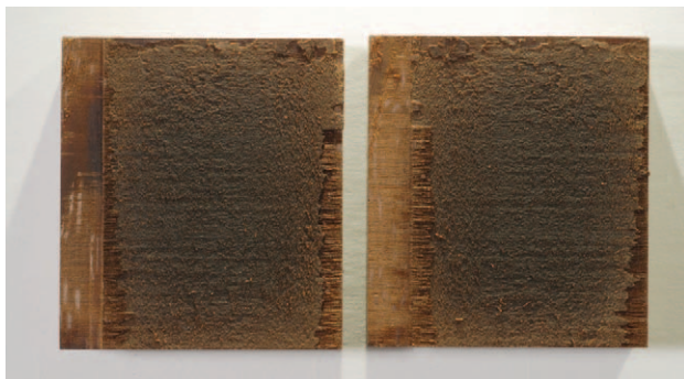
Samples after ASTM D-7247 heat resistant test of an adhesive that still gives wood failure making it likely that the bonded product will pass a fire test (left) and one that does not making it likely that the bonded product will not pass a fire test (right).
