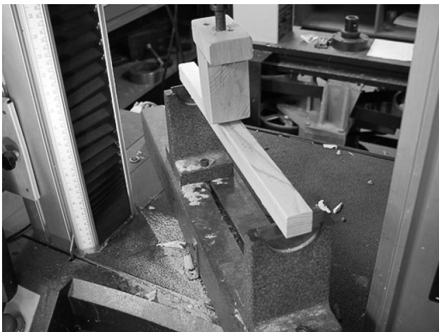
Figure 1.—Testing setup for the flexural tests of small clear samples cut from pentachlorophenol-treated decommissioned utility poles.
