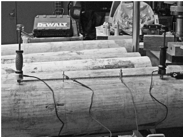
Figure 1.—Locations of moisture meter pins and nails used to measure conductivity and resistance, respectively, in Douglas-fir pole sections treated with pentachlorophenol or copper naphthenate or left untreated.
