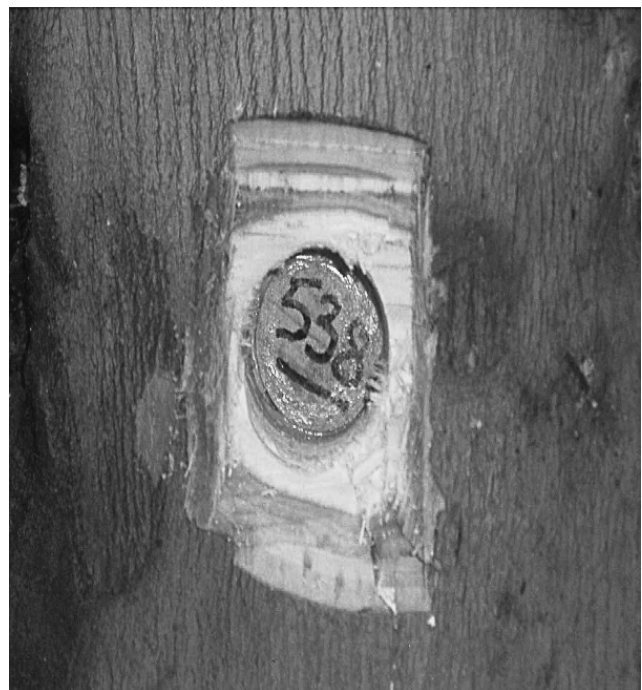
Figure 2.—Identification plug installed.
