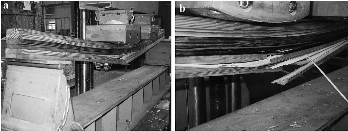
Figure 2.—Bending tests of laminated crossarms made of decommissioned chromated copper arsenate–treated utility pole wood: (a) a laminated beam (Composition C) was tested in two-point loading and (b) failure detail of a laminated crossarm after the bending test.
