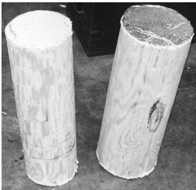
Figure 1.—Pole samples with urethane adhesive and aluminum foil.
