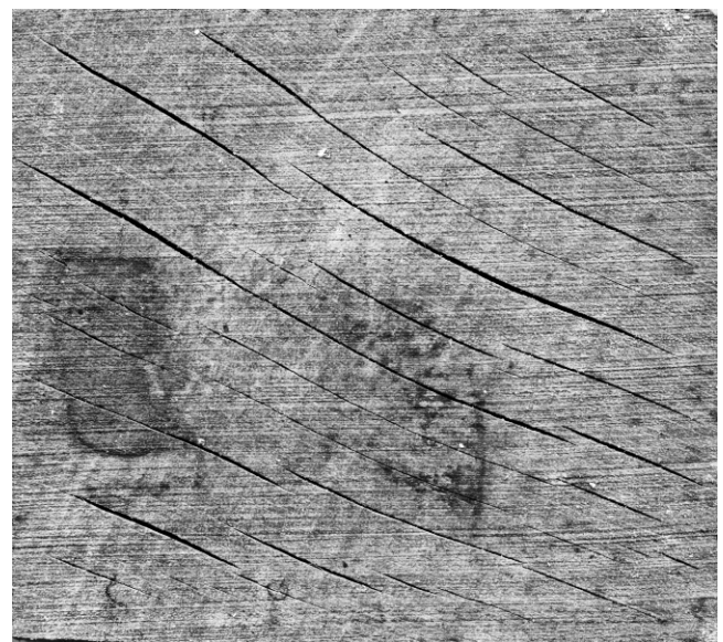
Figure 2.—External pink zone lines on Xylaria polymorpha/Arthrographis cuboidea -inoculated blocks treated with 6.39 \times 10^{-2} kg/m 3 copper sulfate.
