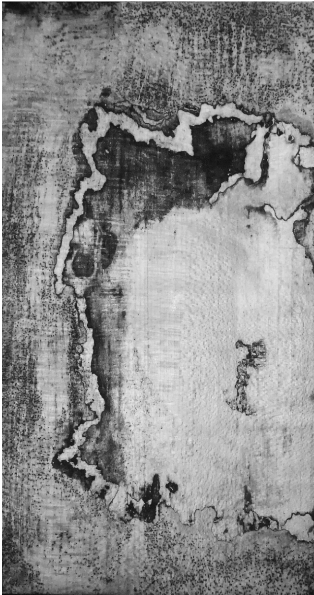
Figure 1.—Sugar maple board treated with a 13 percent solution of copper sulfate and inoculated with Xylaria polymorpha SR001 showing treatment pattern.
