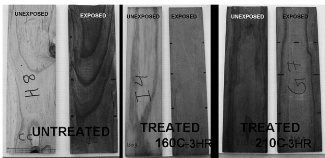
Figure 3.—Comparison of color in unexposed and exposed specimens of after 2,100 hours of accelerated UV weathering. The unexposed and exposed samples belong to the same piece cut from the middle of the thickness of the same specimen.
