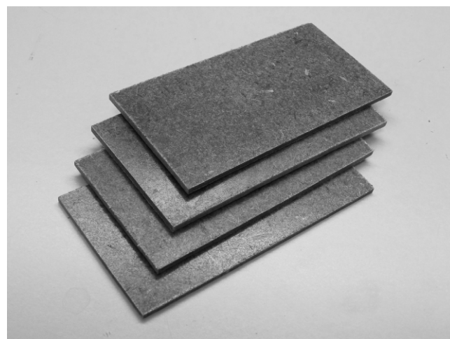
Figure 4.—Kenaf bast fiber bundle/unsaturated polyester composites.
