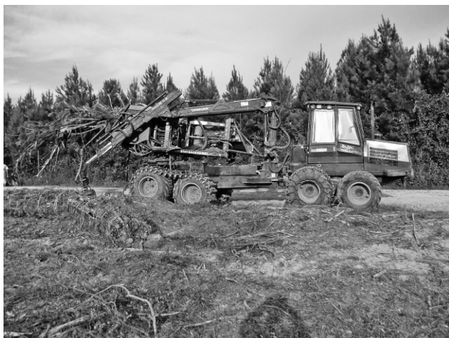
Figure 1.—The John Deere 1490D slash bundler.
