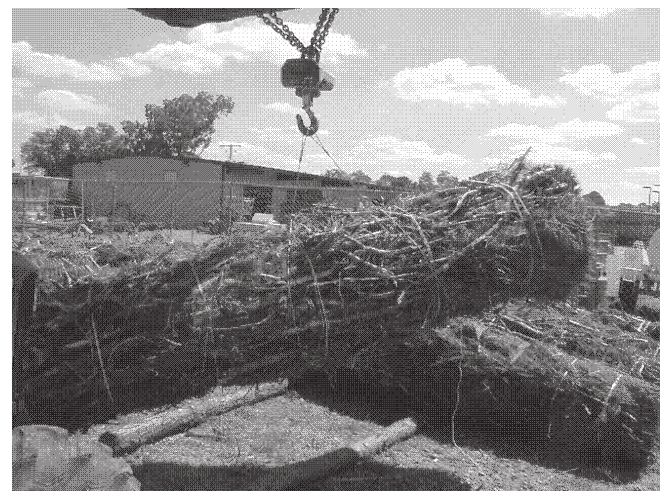
Figure 4.—Weighing slash bundle from pine harvest site in southeastern Arkansas with a crane scales and cables to determine weight change due to exposure.
