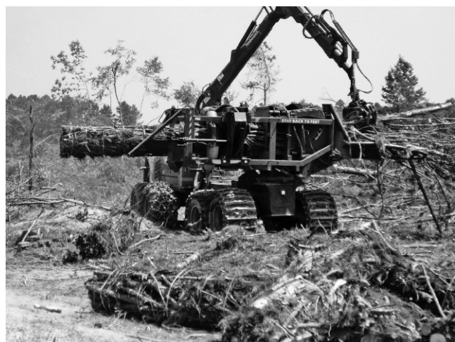
Figure 2.—The John Deere 1490D bundler unit in operation in a pine clear-cut in southeastern Arkansas.
