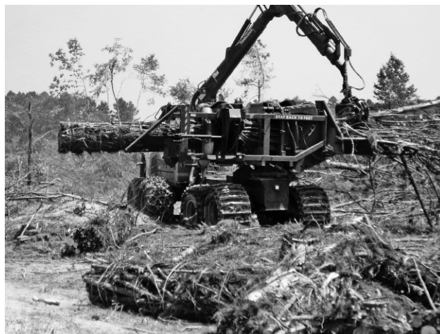
Figure 2.—The John Deere 1490D bundler unit in operation in a pine clear-cut in southeastern Arkansas.
