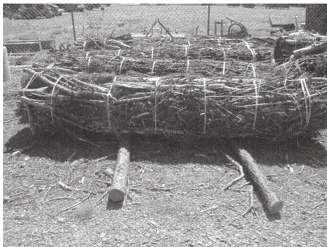
Figure 3.—Study bundles from pine harvest sites in southeastern Arkansas placed on skids for observation and weighing.
