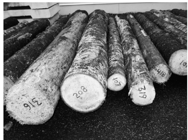
Figure 2.—Examples of the different types of logs included in the study: Log 107, living balsam fir tree, 104 years old; Log 208, balsam fir, dead for 1 year, 110 years old; Log 316, black spruce, dead for 5 years, 88 years old; Log 319, black spruce, dead for 5 years, 86 years old; Log 418, black spruce, dead for 30 years, 185 years old.
