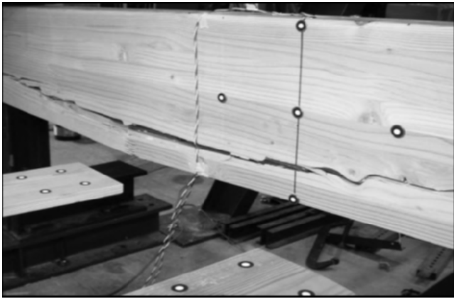
Figure 4.—Reference points at midspan for digital image correlation displacement measurement.
