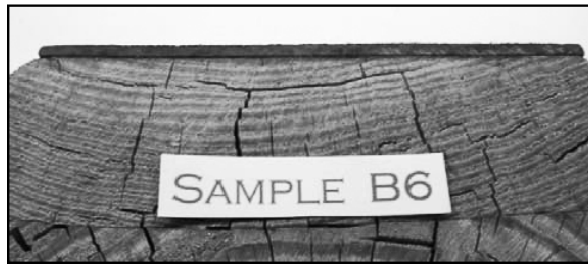
Figure 1.—Cyclic delamination and shear block specimens.
