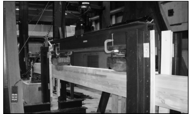
Figure 3.—General view of the four-point bending setup.
