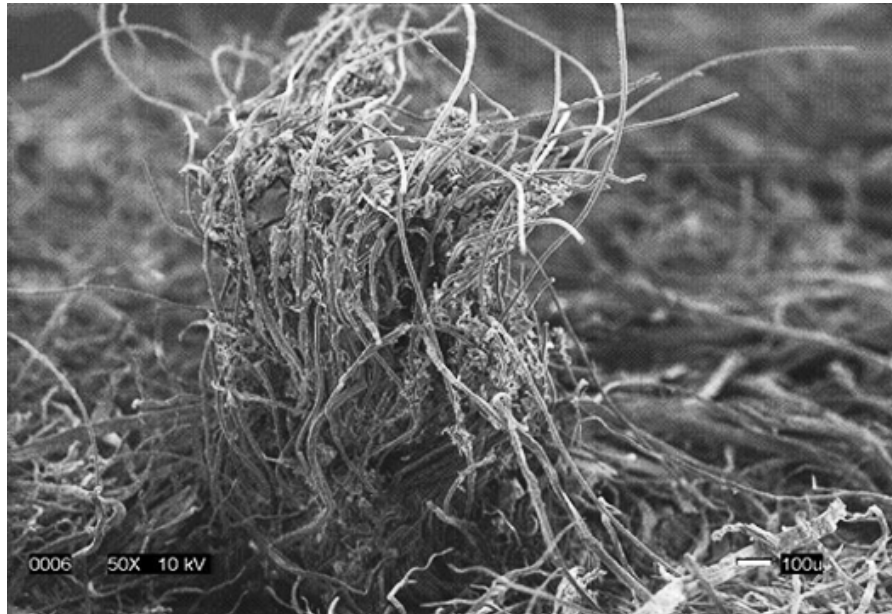
Figure 3.—Fiber tuft protruding from the surface of the wood-fiber core.
