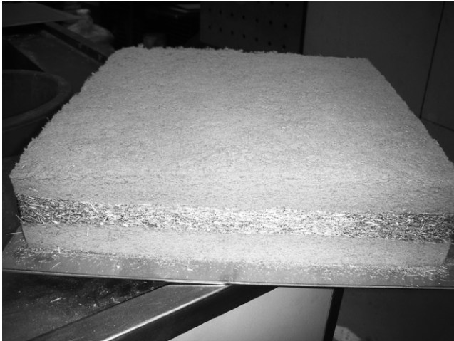
Figure 3.—Unpressed panel mat.
